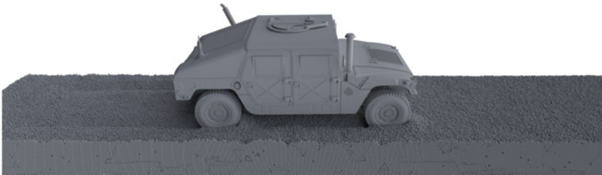
(b) Chrono simulation of vehicle operating on granular/gravel-type material. The motion of every particle in the terrain is monitored by leveraging parallel computing on GPU cards.
