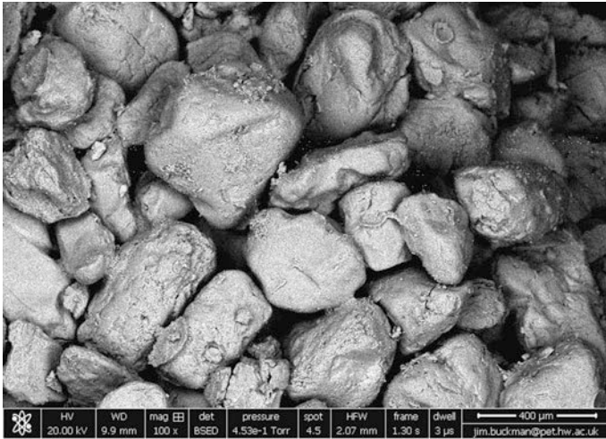
Fig. 1 Sand grains collected from Bédoin, cemented and rimmed with flocculated clay
