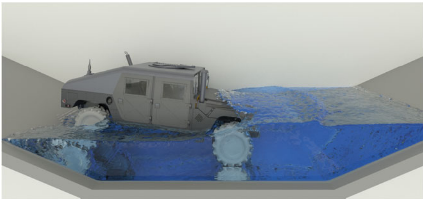
(b) Fording scenario simulated with constraint fluids via Navier-Stokes and SPH. The problem is posed as a set of differential algebraic inclusion equations, see Eq. (8).
